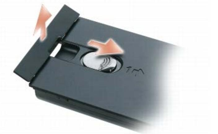
2. Insert the battery straight down into the battery bay.
